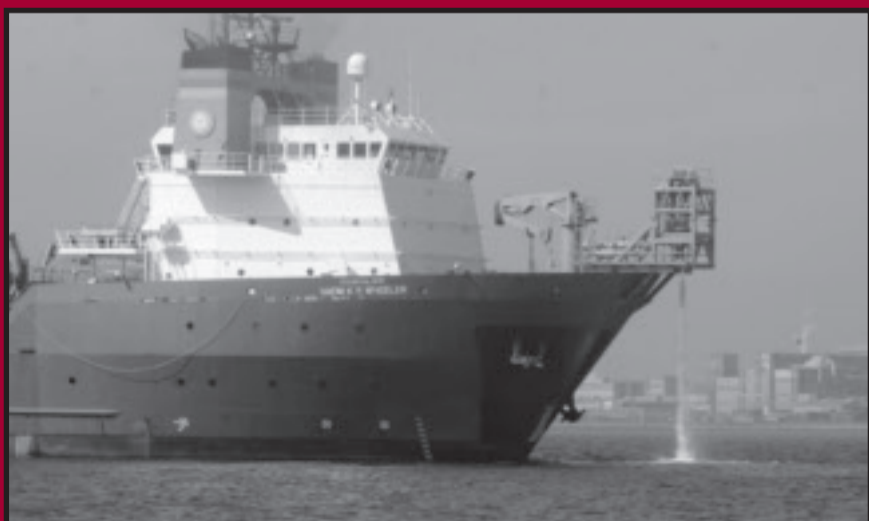
The offshore petroleum distribution system on the USNS Vadm K.R. Wheeler (above) discharges water through pipes aft of the ship as part of the exercise. (U.S. Navy photo by Mass Communication Specialist 3rd Class Madailein Abbott)
